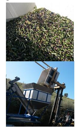
The olives then go through a rinsing process twice (once in a bath on the belt, and again with a spray of water as they come up the belt) as well as an automated sorting process to again help remove any leaves or other debris from the olives.
